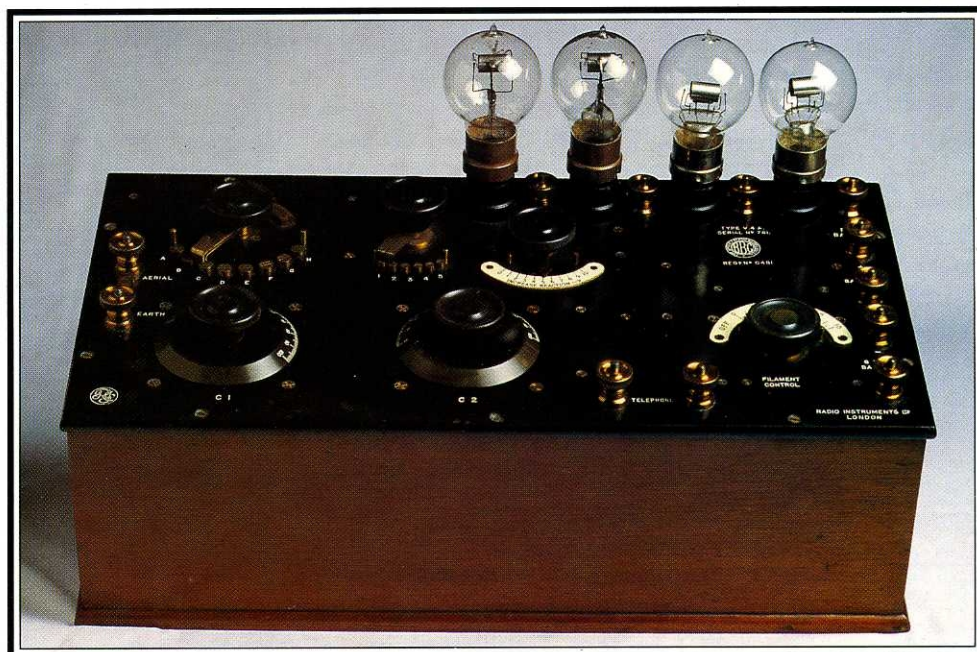
Type V.4.A. 4-valve receiver, made by Radio Instruments Limited of London in 1923
