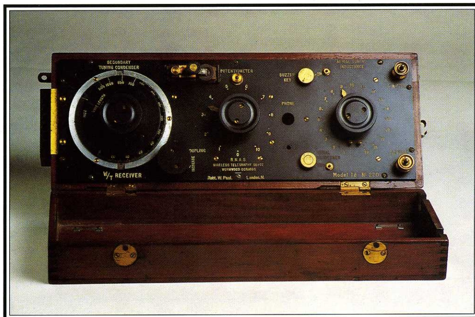
A Crystal W/T Receiver Model Td, manufactured at the Wormwood Scrubs Depot in 1918 for the Royal Naval Air Service
