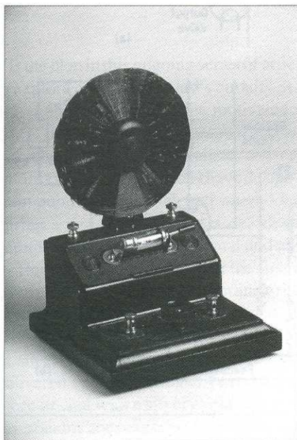
The Brownie Wireless Company's No. 2 Model Crystal Receiver, with plug-in coil attachment for Daventry 5XX (1926)
